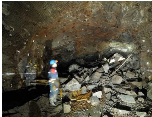
Figure 3: (a) Developed crack on the surface of shotcrete in Test 2 (b) destroyed burden in Test 5 (Shirzadegan et al., 2016b).
