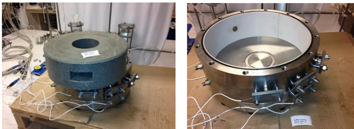
**Figure 20: Photos of the device and the bentonite block used for SH1. One of the cavities can be seen.**
