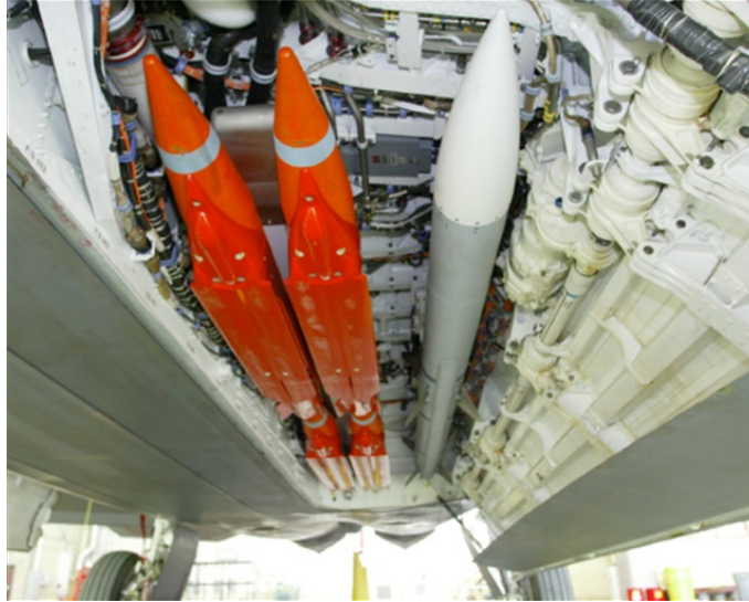
Figure 10: Ordnance for stealth aircraft has to fit in internal bays
