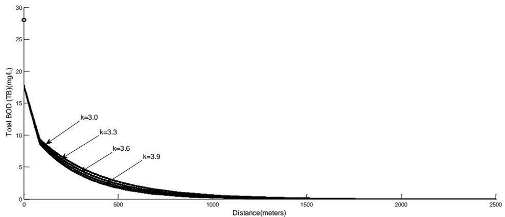
Figure 5: Concentration distribution of total BOD for different values of decay rate of dissolved BOD ( $k$ ).
