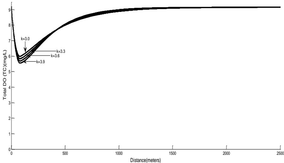
Figure 6: Concentration distribution of total DO for different values of decay rate of dissolved BOD ( $k$ ).
