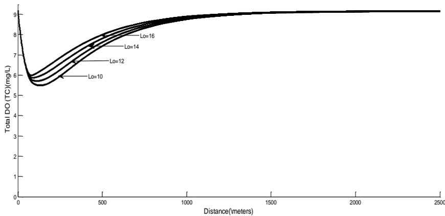
Figure 3: Concentration distribution of Total DO for different values of initial settleable BOD ( $L_0$ )
