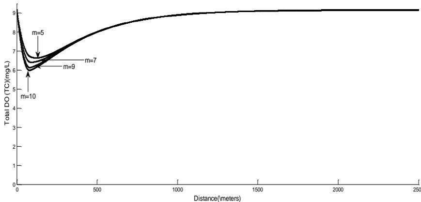
Figure 1: Concentration distributions of total DO for different values of settleable decay rate ( $m$ )
