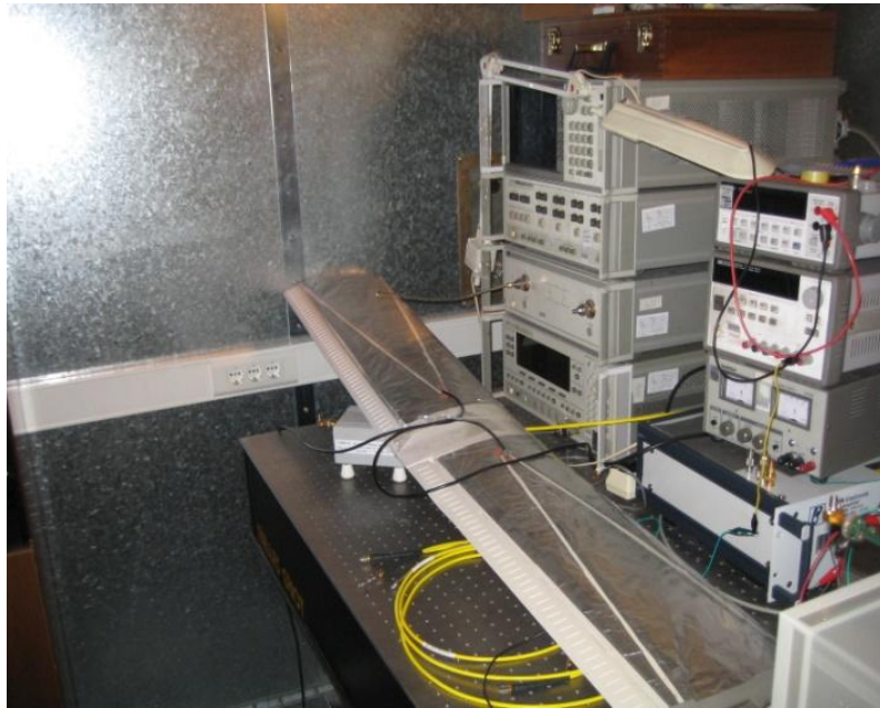
Figure 10. Mounting of the antenna on the wing
