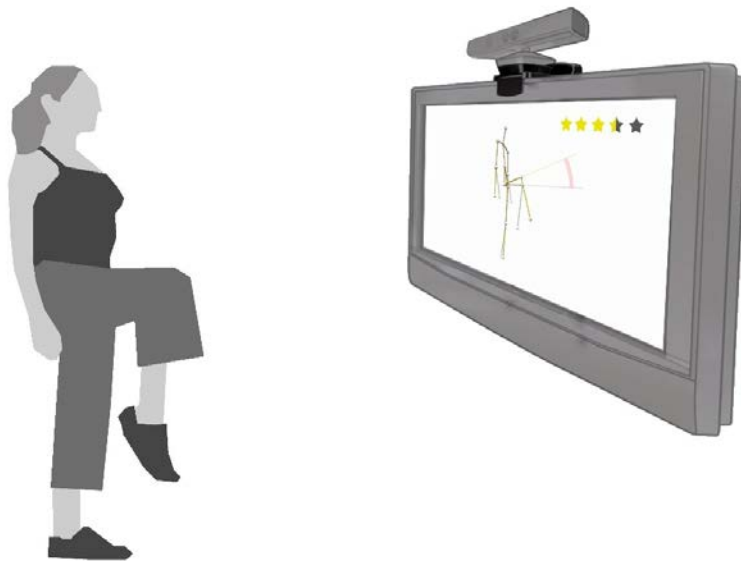
Figure 3: KINOPTIM GUI showing a posture reached by the person and the score translated in stars. The more the stars, the better the achieved posture.
