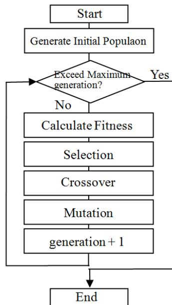
Figure 6-1: The flow of algorithm
