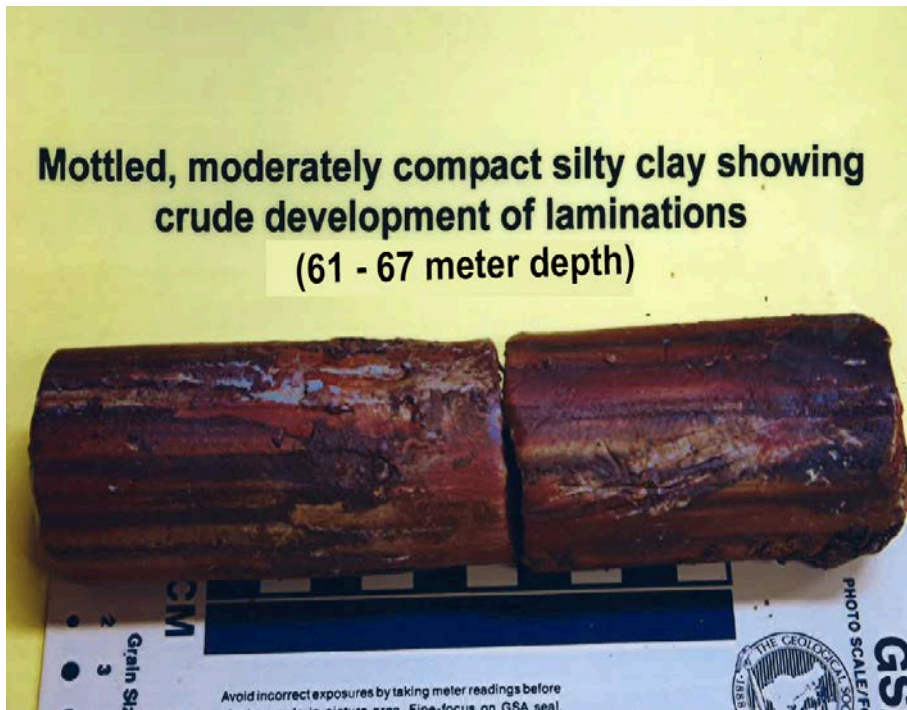
Figure 11: Major lithologic unit above the solid bedrock is dominantly composed of variegated, moderately to highly compact silty clay; often recording higher N or SPT counts. (61 to 67 meter below sea level).
