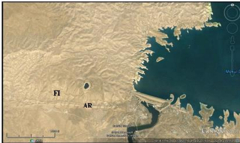
Figure 3: Google Earth image of the Mosul Dam site, located within Butma East anticline. AR = Anticlinal ridge, FI = Flat iron,
