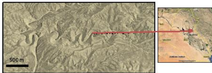
Figure 20: Google Earth image facing NW. Note the acute meanders along the valley indicating possibly a set of sinkholes conjugated together due to side collapsing; forming the valley.
