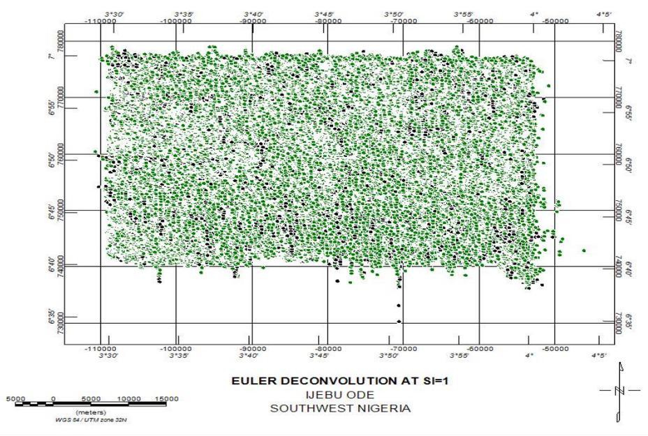
**Figure 9: The Euler Deconvolution at Structural Index of 1**
