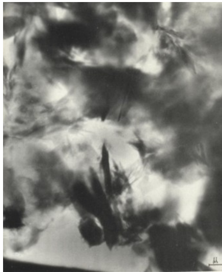
Figure 7: High-voltage transmission electron image of specimen of natural illite clay saturated with water [14]. Various interparticle bond types can be imagined in the coherent clay specimen: Primary chemical bonds, Coulomb electrostatic couplings, shared between sorbed cations, and hydrogen bonds en masse
