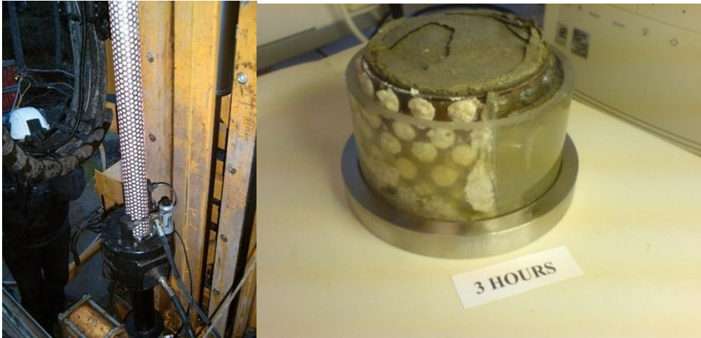
Figure 3: Plug of dense smectite-rich clay confined in perforated copper tube that has been partly coated with mixed talc/clay with the dry mass ratio 3.3/1 and submerged in distilled water for 3 hours. No migration of clay from the tube had occurred from the coated part while penetrated clay had begun to embed the tube in the uncoated part.
