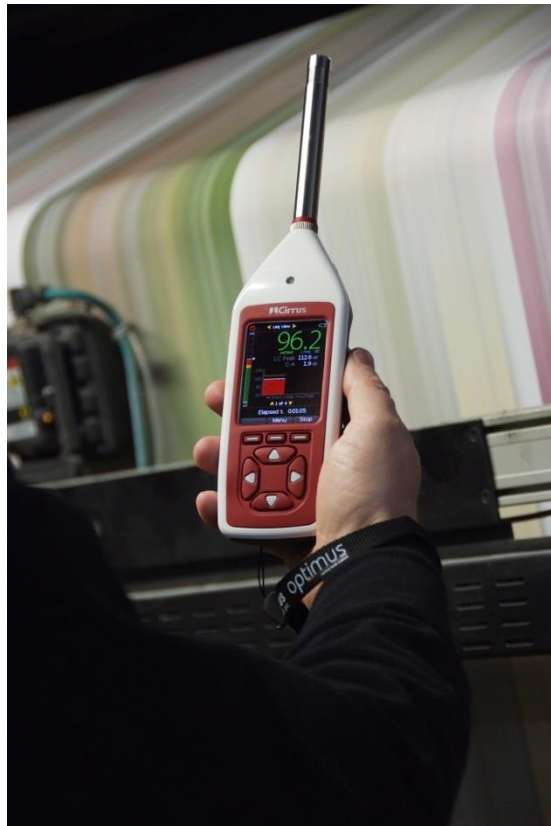
Figure 9: A typical sound level meter (Source: Cirrus Research Plc, 2015)
