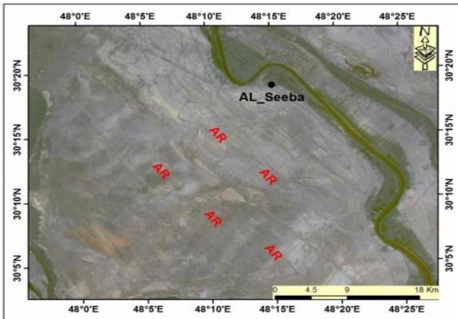
**Figure 12: Satellite image showing abandoned river courses (AR) of Shat Al-Arab due to the growth of Siba subsurface anticline.**
