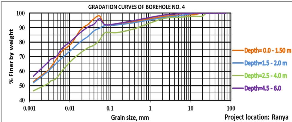
Figure 6: Gradation curve of borehole (No.4) Ranya area.
