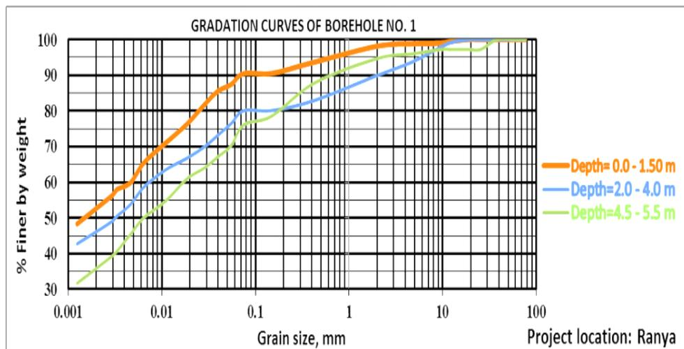
**Figure 3: Gradation curve of borehole (No.1) Ranya area.**
