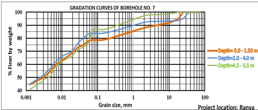
Figure 9: Gradation curve of borehole (No.7) Ranya area.
