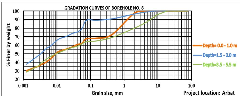
Figure 18: Gradation curve of borehole (No.8) Arbat area.
