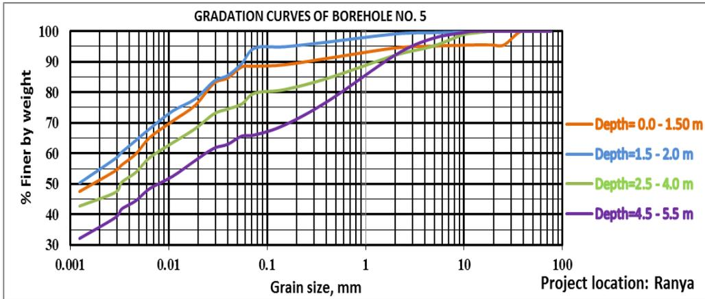
Figure 7: Gradation curve of borehole (No.5) Ranya area.
