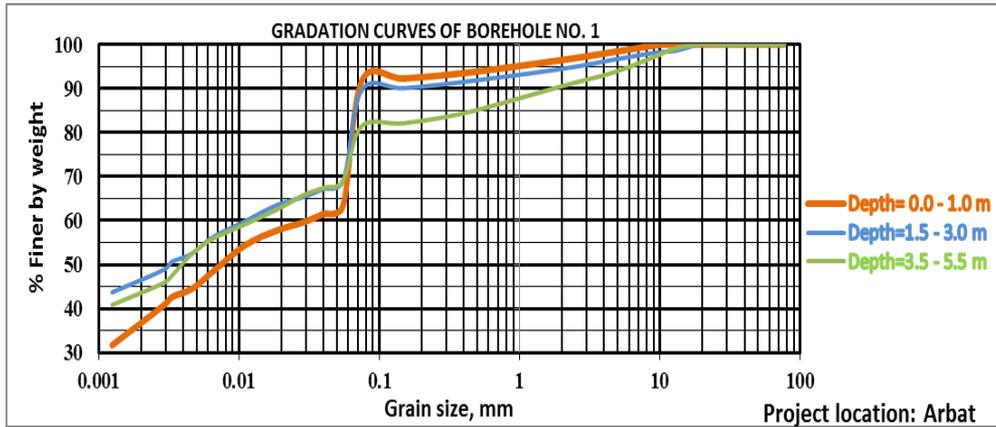
Figure 11: Gradation curve of borehole (No.1) Arbat area.
