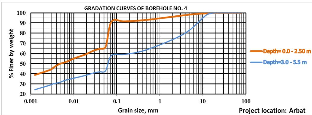
Figure 14: Gradation curve of borehole (No.4) Arbat area.
