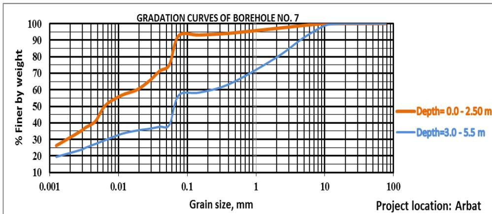
Figure 17: Gradation curve of borehole (No.7) Arbat area.
