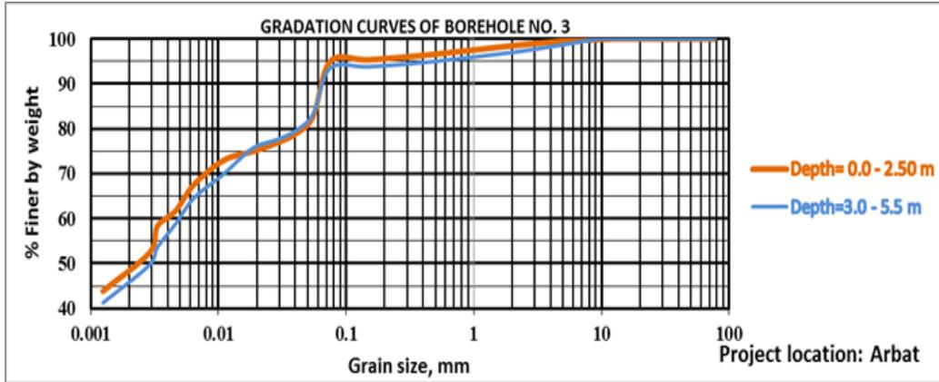
Figure 13: Gradation curve of borehole (No.3) Arbat area.
