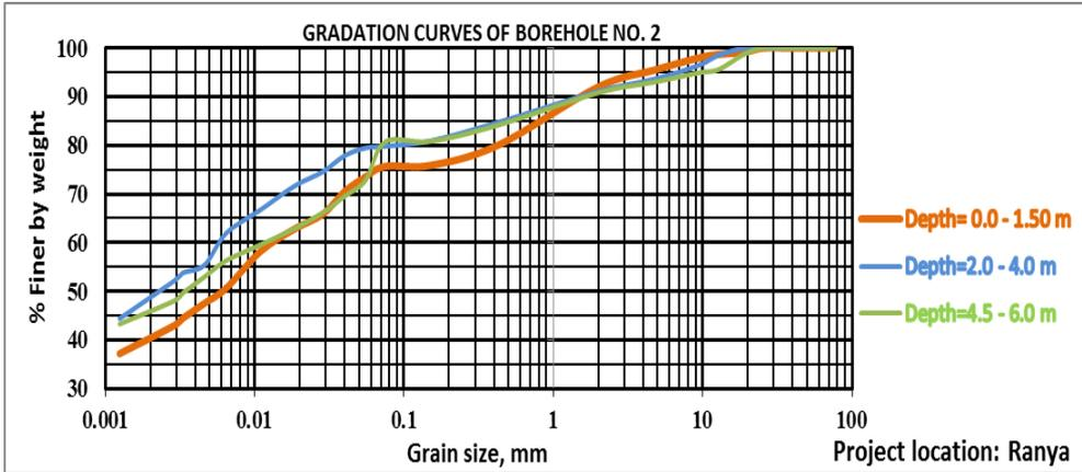
Figure 4: Gradation curve of borehole (No.2) Ranya area.
