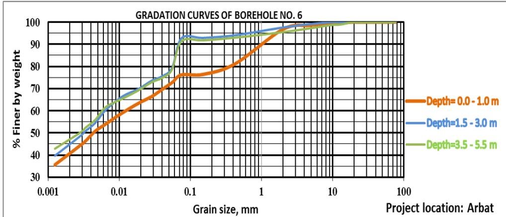
Figure 16: Gradation curve of borehole (No.6) Arbat area.
