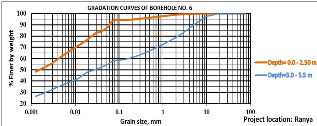
Figure 8: Gradation curve of borehole (No.6) Ranya area.
