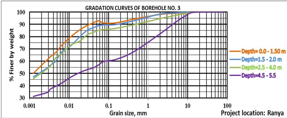
Figure 5: Gradation curve of borehole (No.3) Ranya area.
