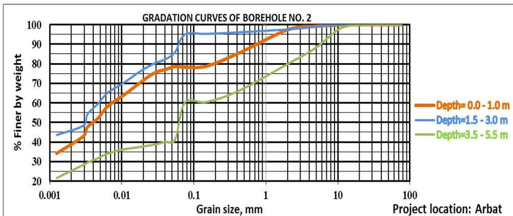
Figure 12: Gradation curve of borehole (No.2) Arbat area.
