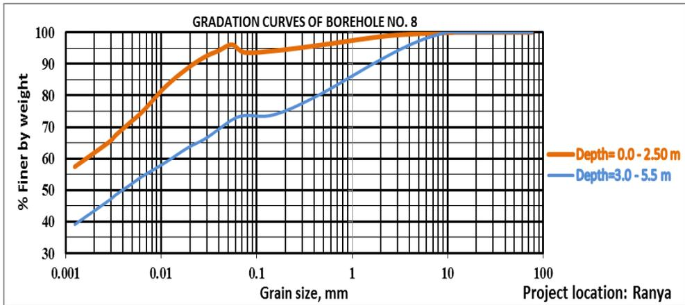
Figure 10: Gradation curve of borehole (No.8) Ranya area.
