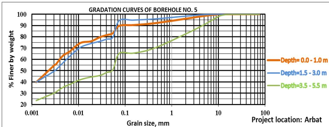
Figure 15: Gradation curve of borehole (No.5) Arbat area.
