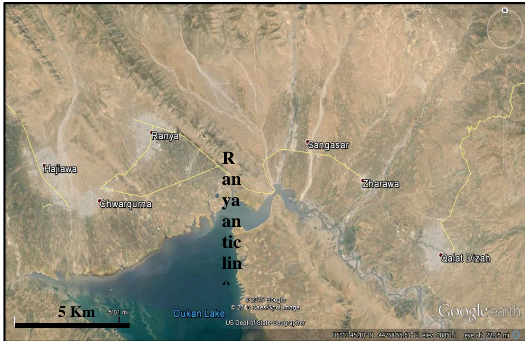
Fig.10: Google Earth image showing the huge alluvial fans that have supplied the soft materials forming the claystone and sandstone beds within the Dokan Conglomerate. Note the absence of a large part of the southwestern limb; east of ChwarQurna town, most probably due to normal faulting that runs parallel to the western bank of Dokan lake.
