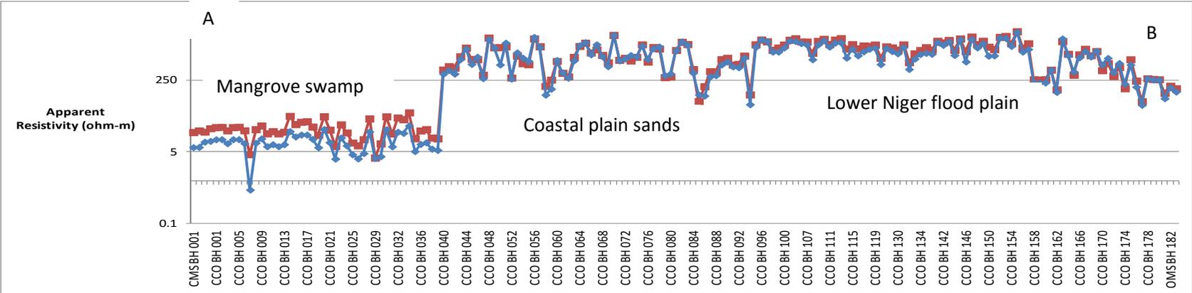
Fig. 10: Apparent Resistivity of surface layers (0-10m) along the traverse in the Eastern Niger delta
