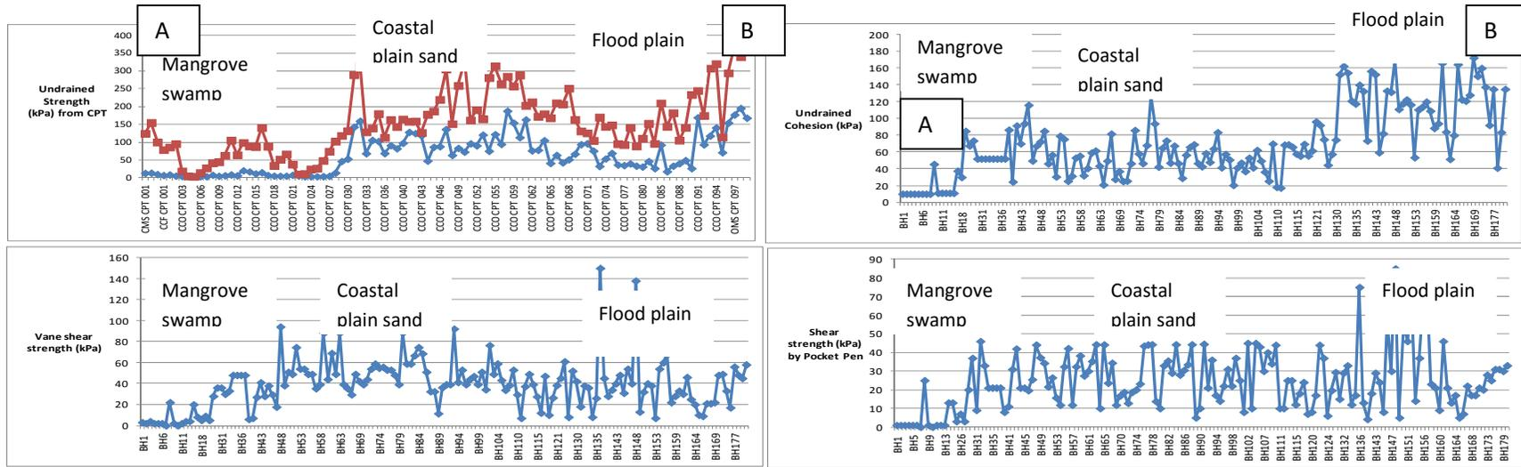
Fig. 12: Average undrained strength (0-10m) from CPT, Triaxial test, Vane and Pocket Penetrometer along the traverse in the Eastern Niger delta
