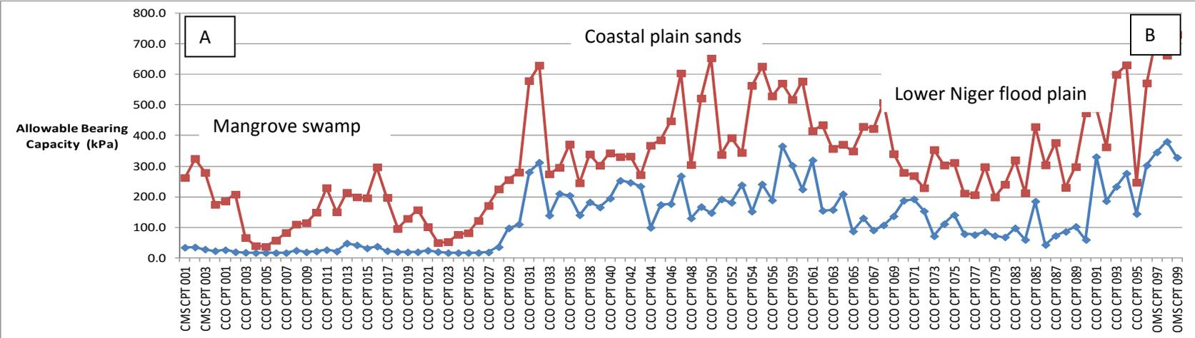
Fig. 17: Allowable Bearing Pressure along the traverse in the Eastern Niger delta derive from CPT
