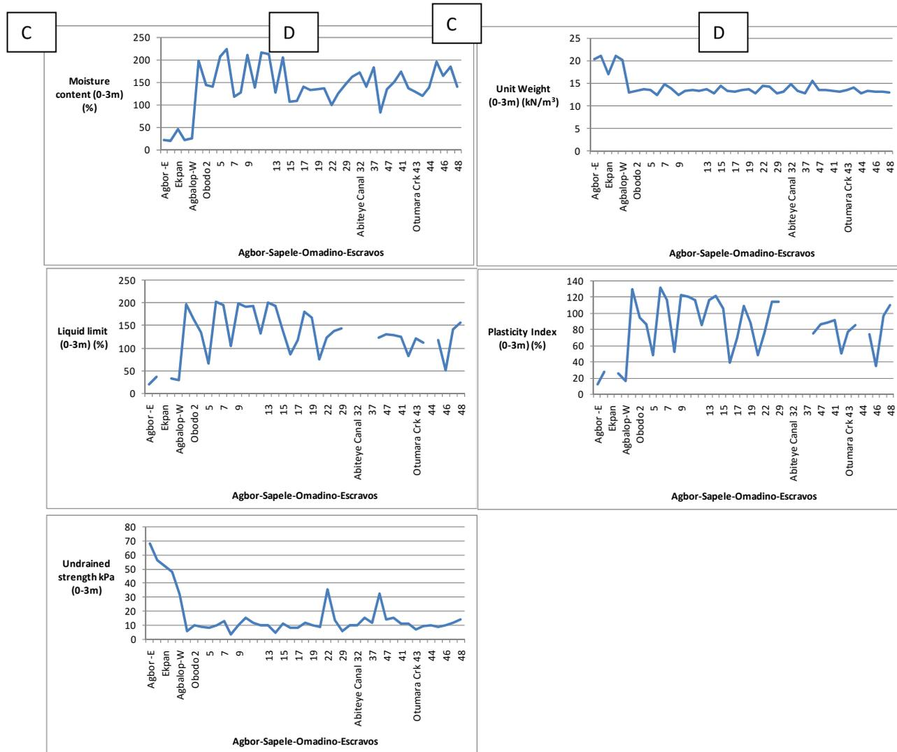
Fig. 14: Geotechnical properties along the traverse in the Western Niger delta
