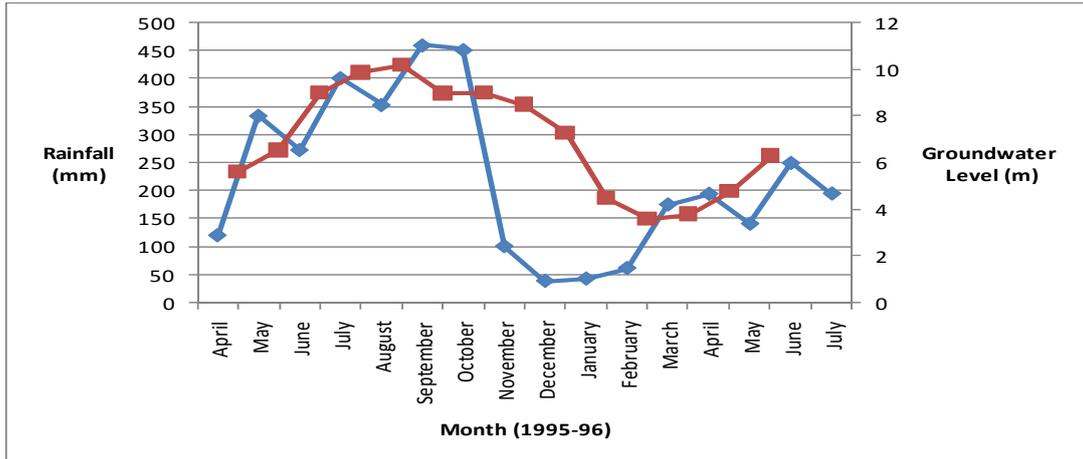
Fig. 9: Rainfall distribution and groundwater level response in the Niger delta
