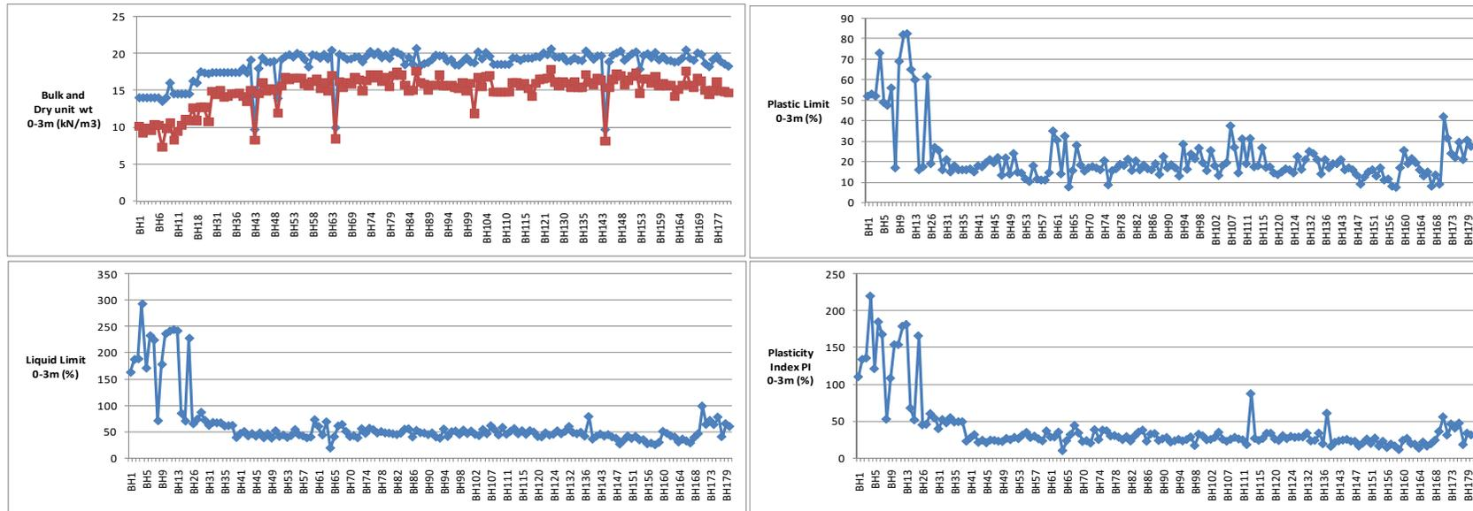
Fig. 16: Bulk unit weight and Atterberg's limits along the traverse in the Eastern Niger delta
