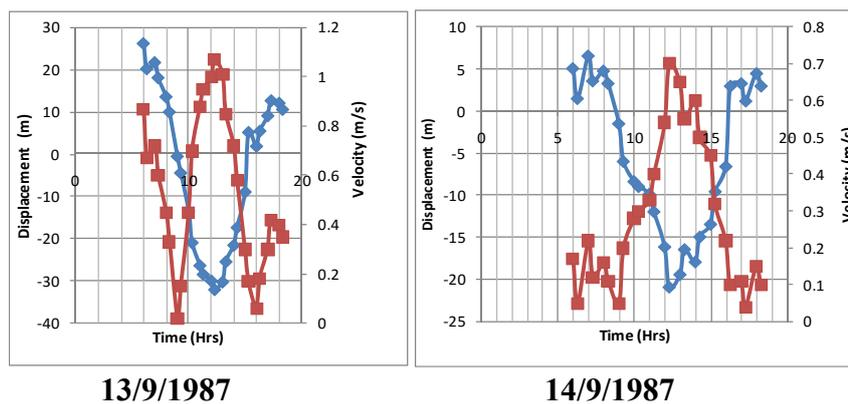
Fig.4: Variation in average tidal velocities and flow displacement in Imo River
