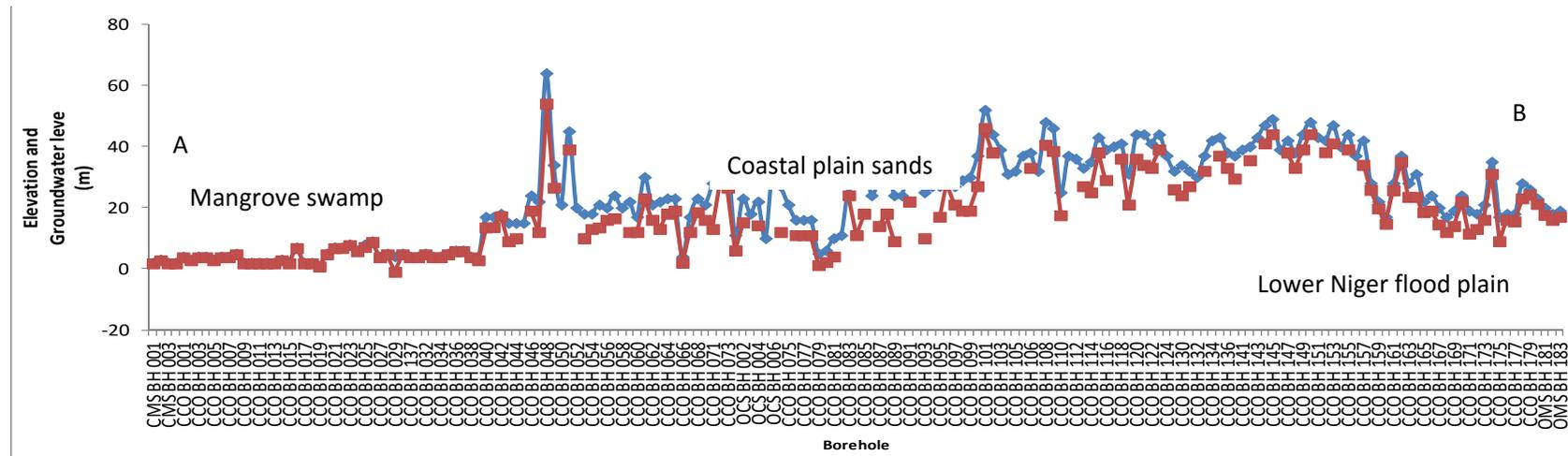
Fig. 8: Groundwater surface elevation along the traverse in the Eastern Niger delta
