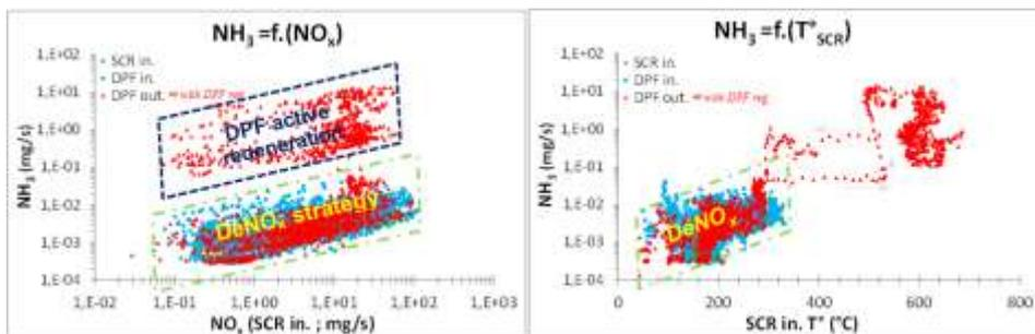
Figure 11. CADC hot w/wo DPF reg. -  $\text{NH}_3$  slip (DPF out.)= f. ( $\text{NO}_x$  abatement &  $T^\circ\text{SCR in.}$ )
