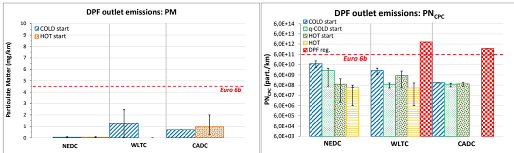
Figure 19. Particulate Matter (PM) and Particle Number (PN)
