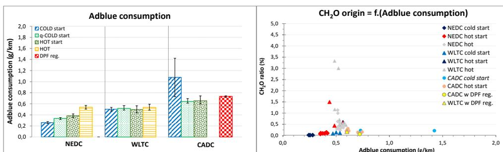
Figure 17. Estimated AdBlue consumption/cycle (left graph) & AdBlue's maximum potential contribution to  $\text{CH}_2\text{O}$  (right graph)
