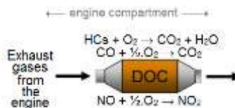
Figure 1. Schematic diagram of DOC functioning
