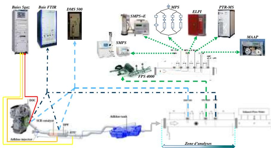
Figure 4. Diagram of the exhaust line and analyzers samplings
