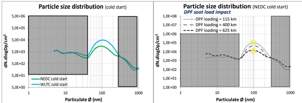
Figure 20. Mean particle size distribution during cold cycles without DPF regeneration
