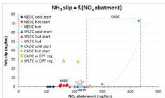
Figure 12.  $\text{NH}_3$  slip (DPF out.)=  $f.(\text{NO}_x \text{ DPF out.} - \text{NO}_x \text{ SCR in.})$
