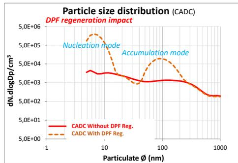
Figure 21. Particles size distribution (CADC, w/w/o DPF regeneration)
