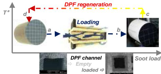
Figure 3. Schematic diagram of DPF loading and cleaning
