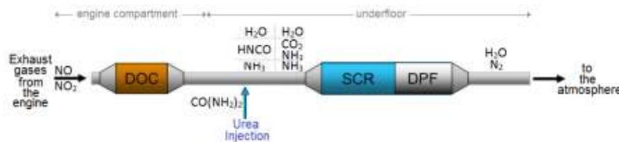
Figure 2. Schematic diagram of SCR catalyst functioning
