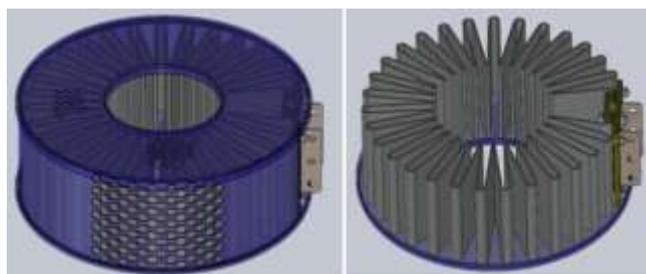
Figure 4: Active filter cartridge, flow from outside to inside
