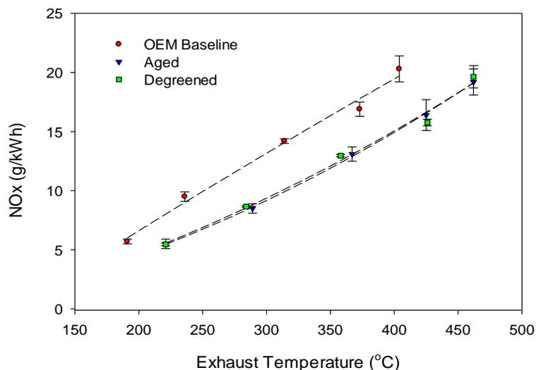
Figure 7: Nitrogen oxides emissions vs. exhaust temperature
