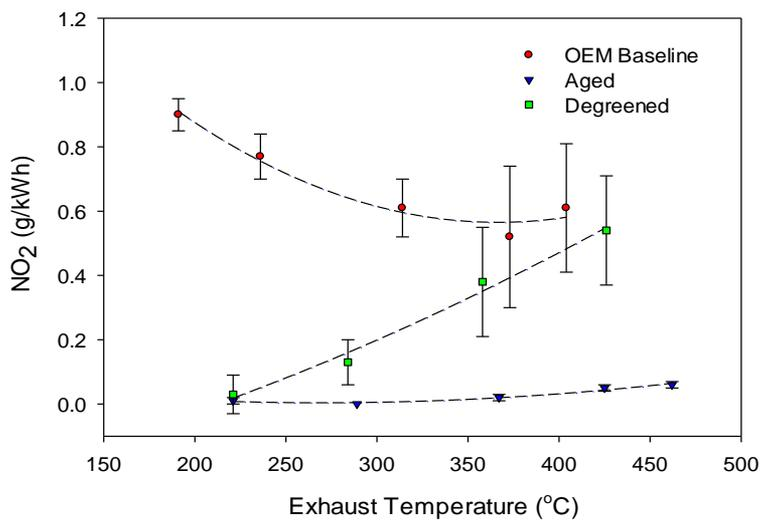
Figure 6: Nitrogen dioxide emissions vs. exhaust temperature
