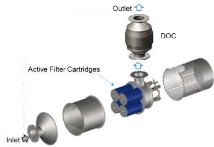
Figure 2: Exploded view of an Active Diesel Particulate Filter (ADPF)
