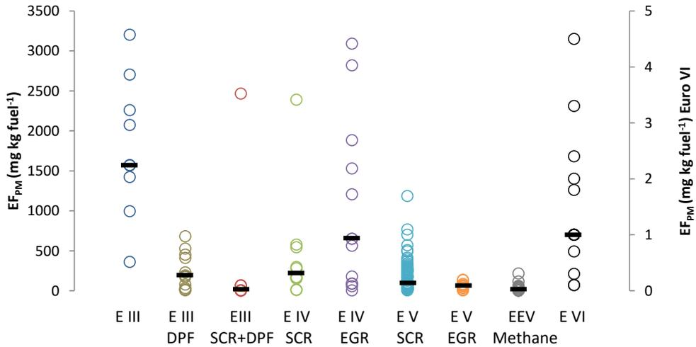
Figure 4. Measured  $EF_{PM}$  from all buses by Euro standard/aftertreatment system (circles) and median  $EF_{PM}$  (black lines). The secondary axis is for Euro VI.
