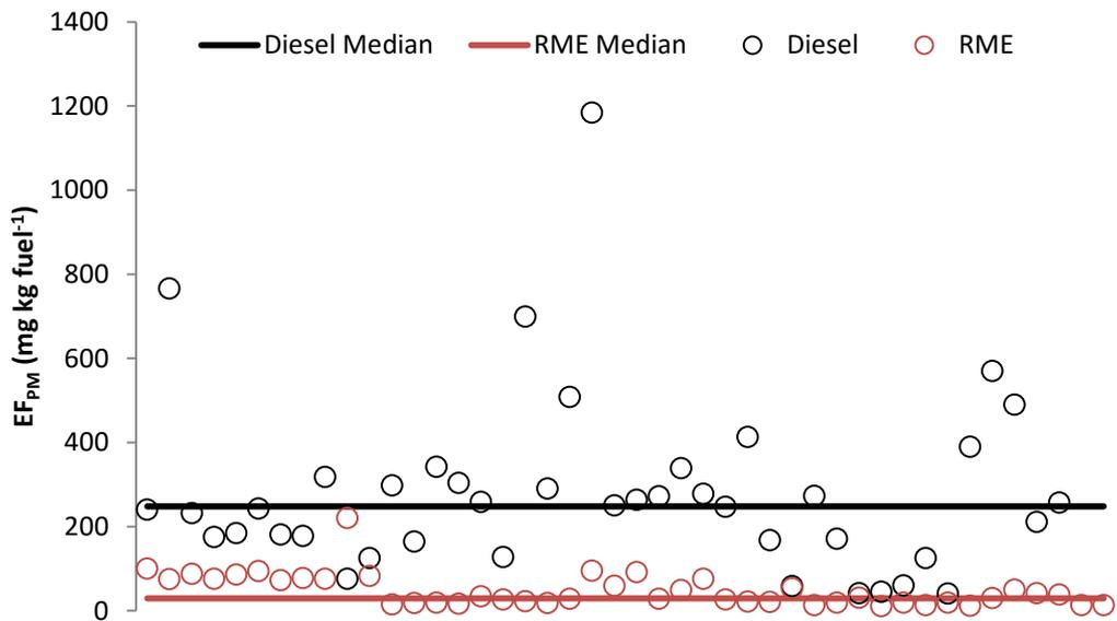
Figure 7. Median EF<sub>PM</sub> for Euro V busses running on RME (red symbols) and diesel (black symbols).
