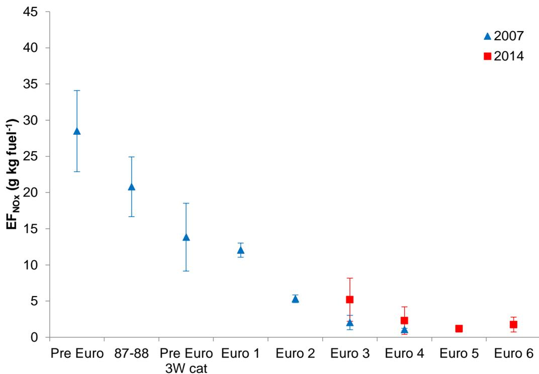
Figure 13. NO<sub>x</sub> emissions from gasoline cars as measured in Gothenburg 2007 and 2014.
