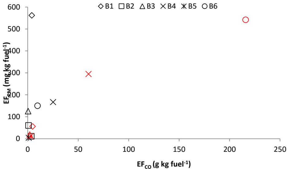
Figure 9.  $EF_{PM}$  for buses that have been tested at multiple years and where there has been a fuel switch (red symbols are  $EF_{PM}$  when fueled with RME).
