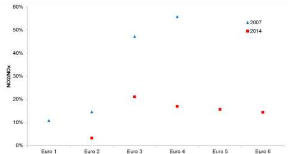
Figure 16.  $\text{NO}_2/\text{NO}_x$  ratio in exhausts from diesel cars as measured in Gothenburg 2007 and 2014.
