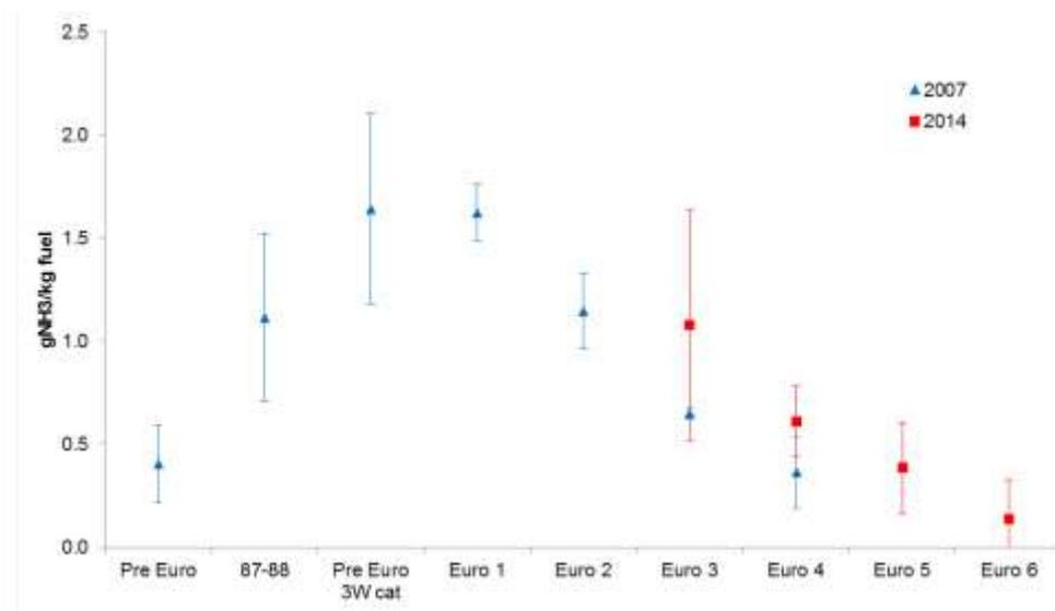
Figure 14. NH<sub>3</sub> emissions from diesel cars as measured in Gothenburg 2007 and 2014.
