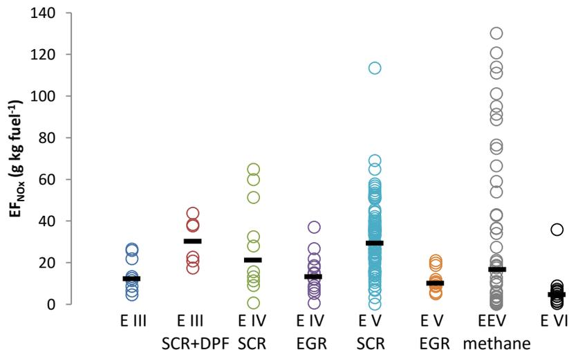
Figure 2. Measured  $EF_{NOx}$  from all buses by Euro standard and aftertreatment system (circles) and median  $EF_{NOx}$  (black lines).
