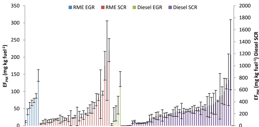
Figure 6. EF<sub>PM</sub> of the tested Euro V buses with respect to fuel and NO<sub>x</sub> abatement technology. The secondary y-axis is for Diesel SCR buses. Stated errors are at the statistical 95% confidence level.
