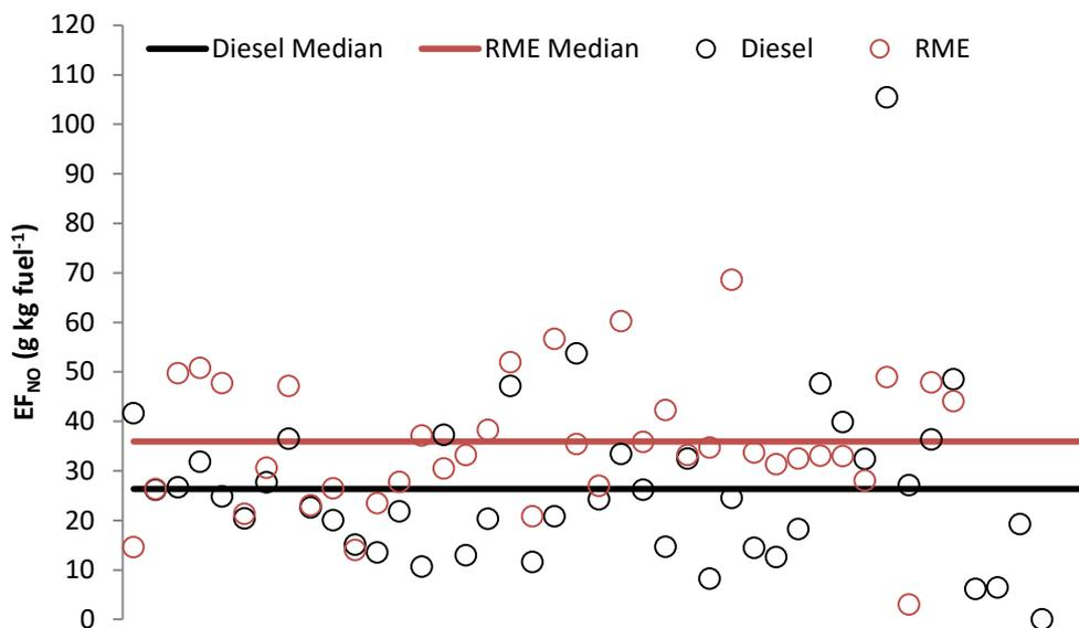
Figure 8. Median  $EF_{NO}$  for Euro V busses running on RME (red symbols) and diesel (black symbols).
