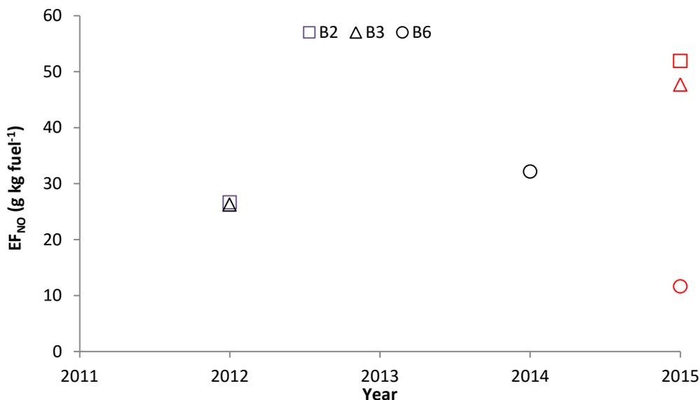
Figure 10. EF<sub>NO</sub> for buses that have been tested at multiple years and where there has been a fuel switch (red symbols are EF<sub>NO</sub> when fueled with RME).
