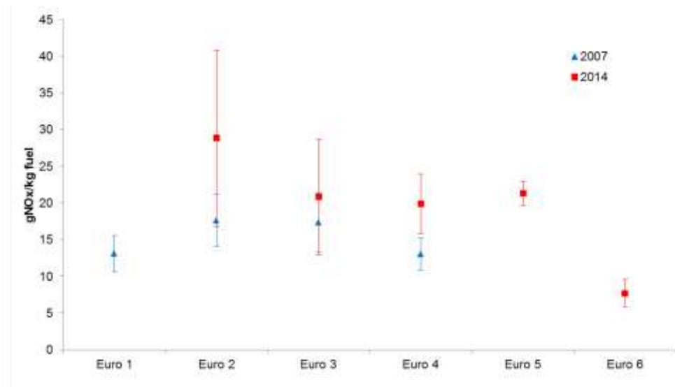
Figure 15. NO<sub>x</sub> emissions from diesel cars as measured in Gothenburg 2007 and 2014.
