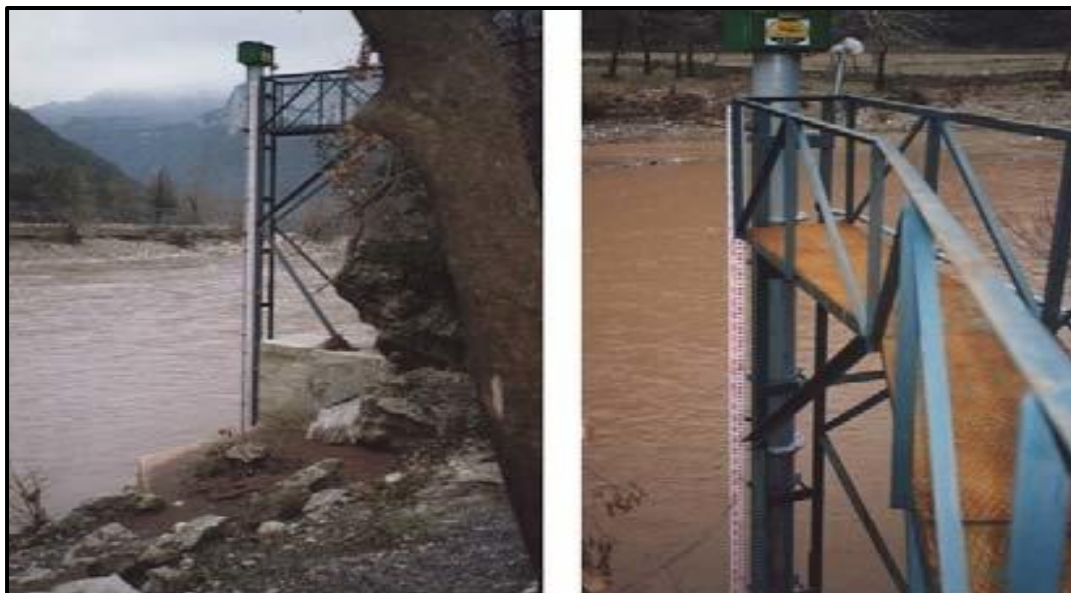
Figure 4: Water level staff gauge at Kovali Dam, and at Sultan reed fields, Kayseri, Turkey [9].
