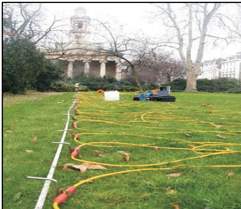
Figure 6: Typical array of electrodes for ERT RSK electrical resistivity imaging [33].
