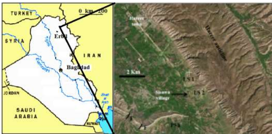
Figure 1: Flash Earth image of Hareer anticline. LS 1 and LS 2 = Landslide No. 1 and 2, PSh = Northwestern plunge of Shakrook anticline, F = fault
