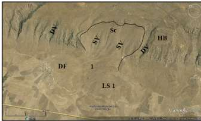
Fig.12: Google Earth image facing NW. Note Sisawa Landslide No.1 (LS 1), the debris flow (DF), shell-like scar (Sc), and the hanging block (HB), which forms daylight slope. SV = Shallow valley, DV = Deep valley. Limits of the shell-shaped scar.
