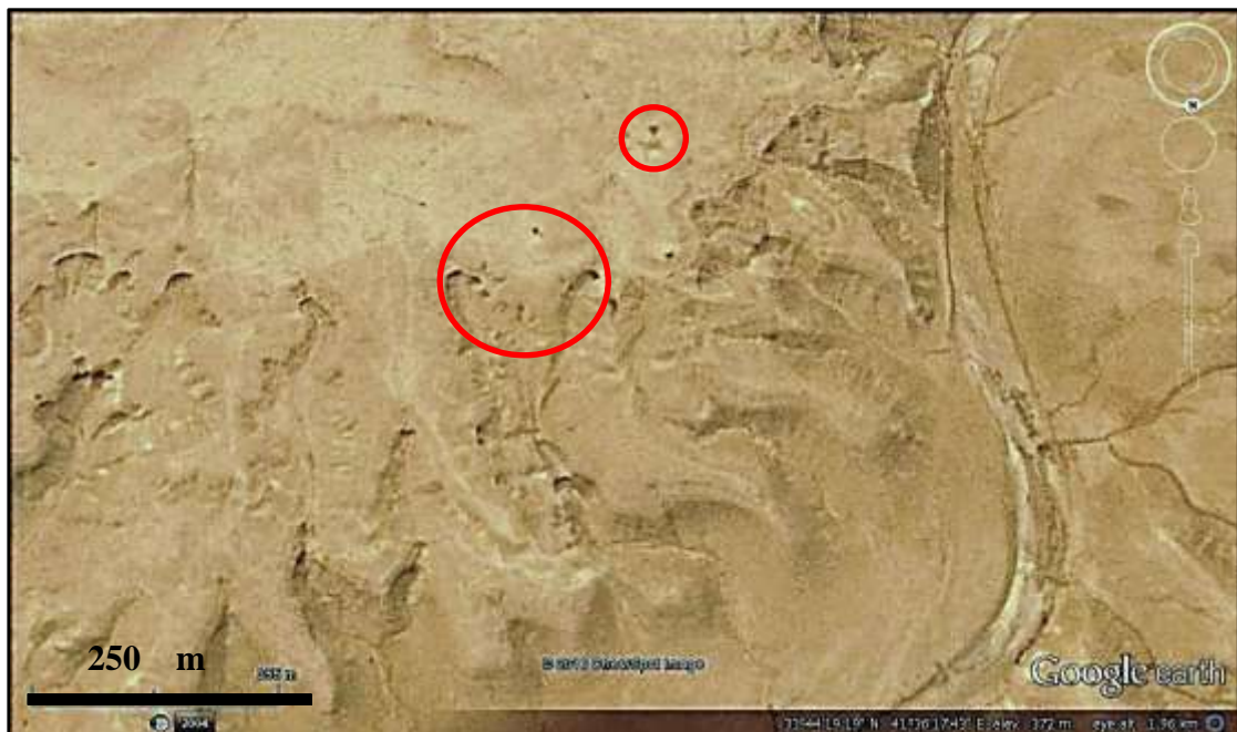
Figure 7: Google Earth image showing sinkholes in Part 4
