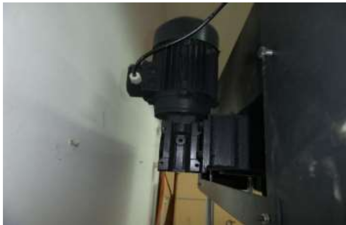
Fig. 6: Three – phase motor.
