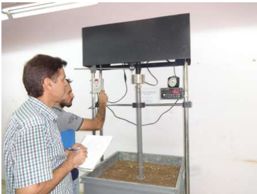
Fig. 9: Carrying out cyclic load test.
