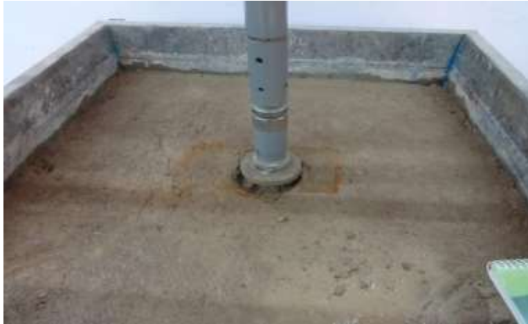
Fig. 7: Model footing connected to the transfer arm.
