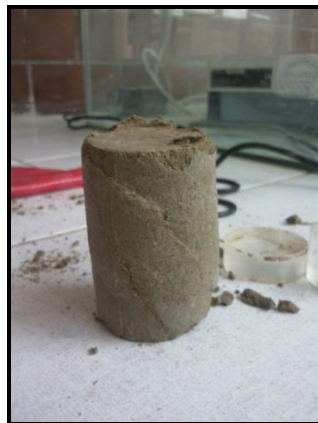
Figure 3: Failure of samples of compacted stabilized soil after triaxial testing
