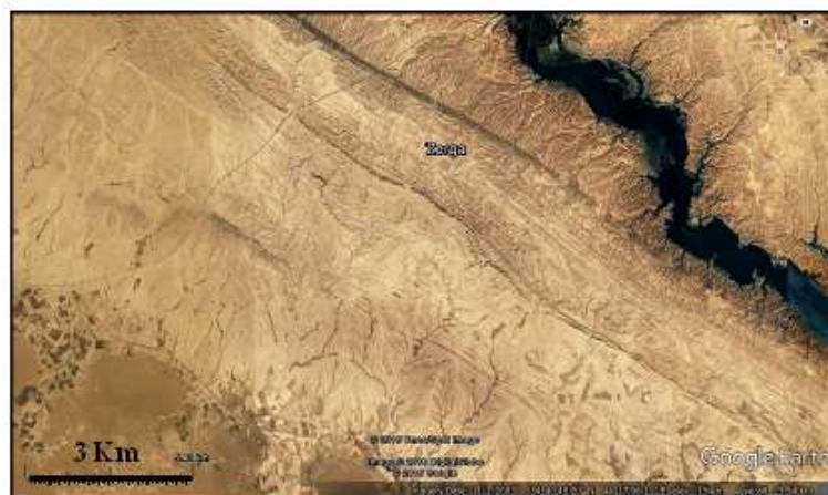
Figure 3: Google Earth Image showing Bajada along Himreen North anticline and dendritic drainage pattern
