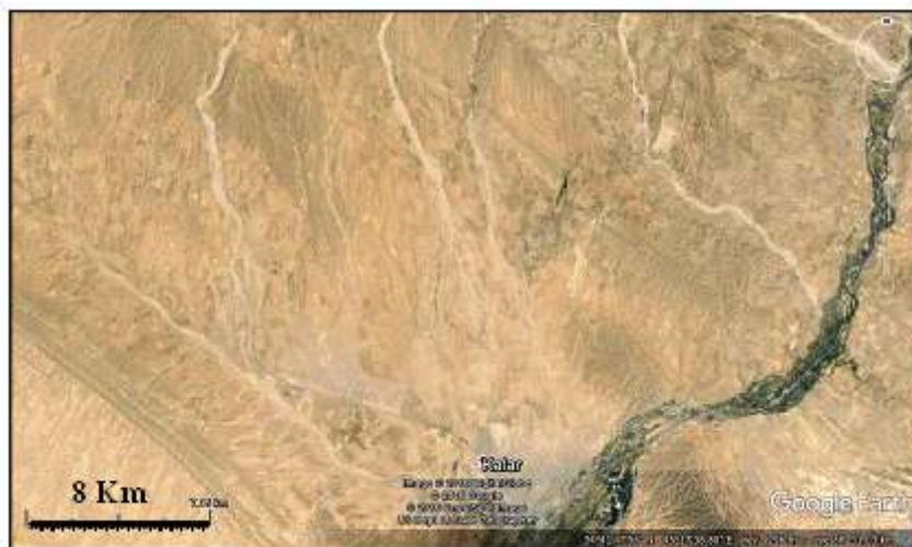
Figure 4: Google Earth image showing parallel drainage pattern (in the lower reaches) and dendritic pattern (in the upper reaches), north of Kalar town
