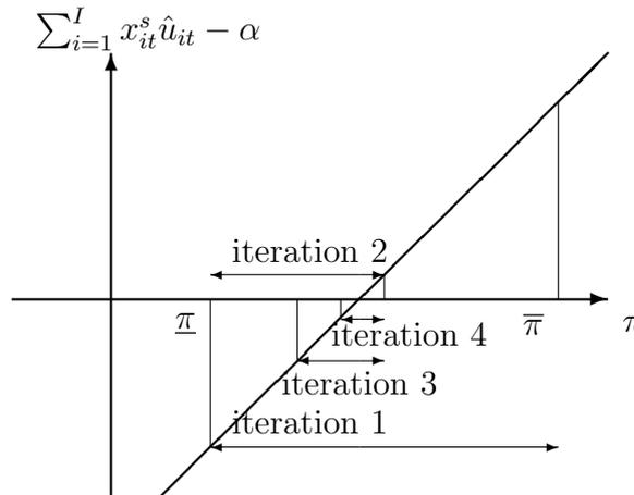
Figure 6: Binary search in lambda iteration
