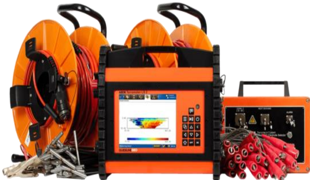
Figure 1: ABEM Terrameter and its accessories (Pacanowski et al. , 2022).
