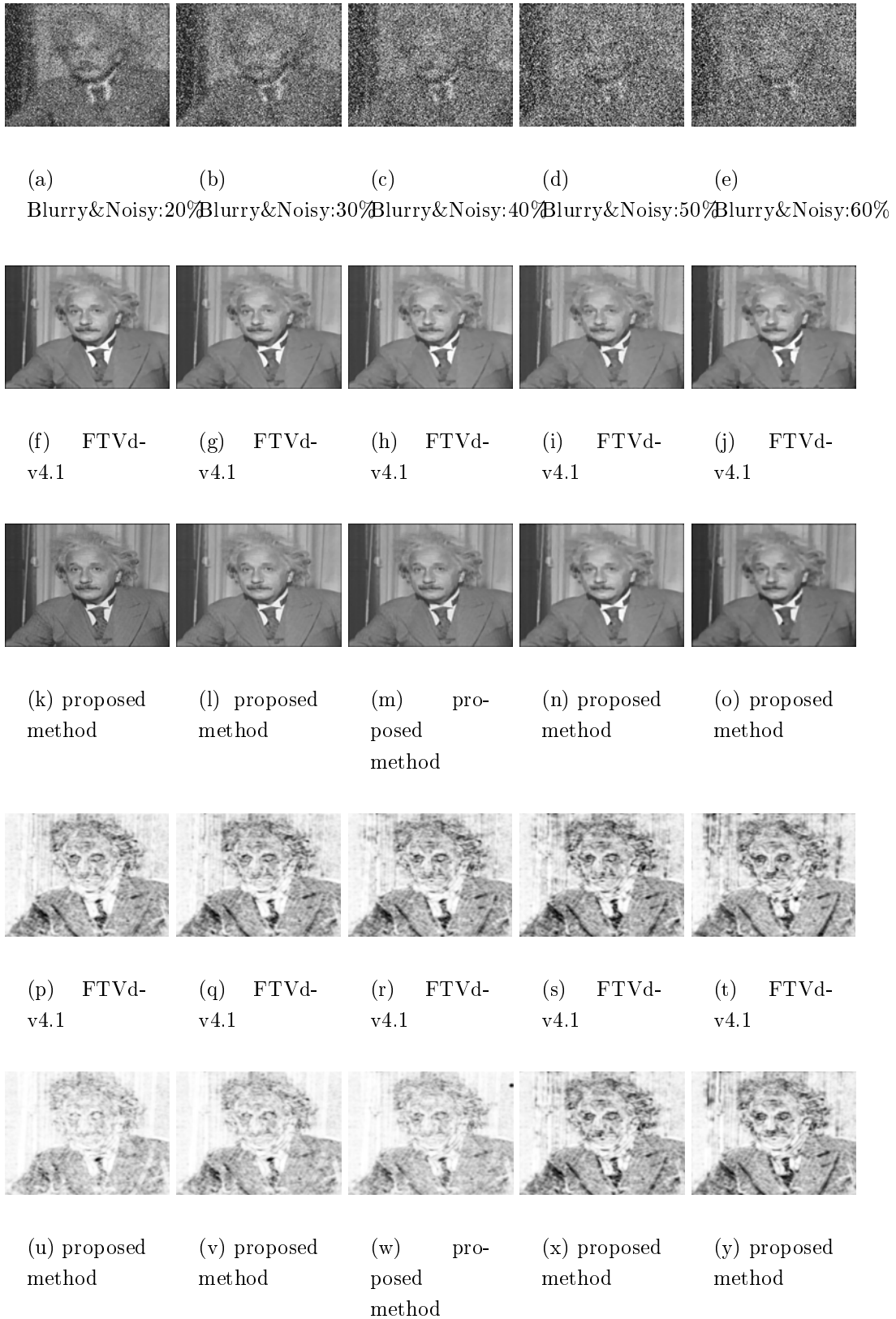
Figure 3: Recovered images of different methods on the Einstein image corrupted by Gaussian blur G([7, 7], 5) and salt-and-pepper noise with noise levels from 20% to 60%.
