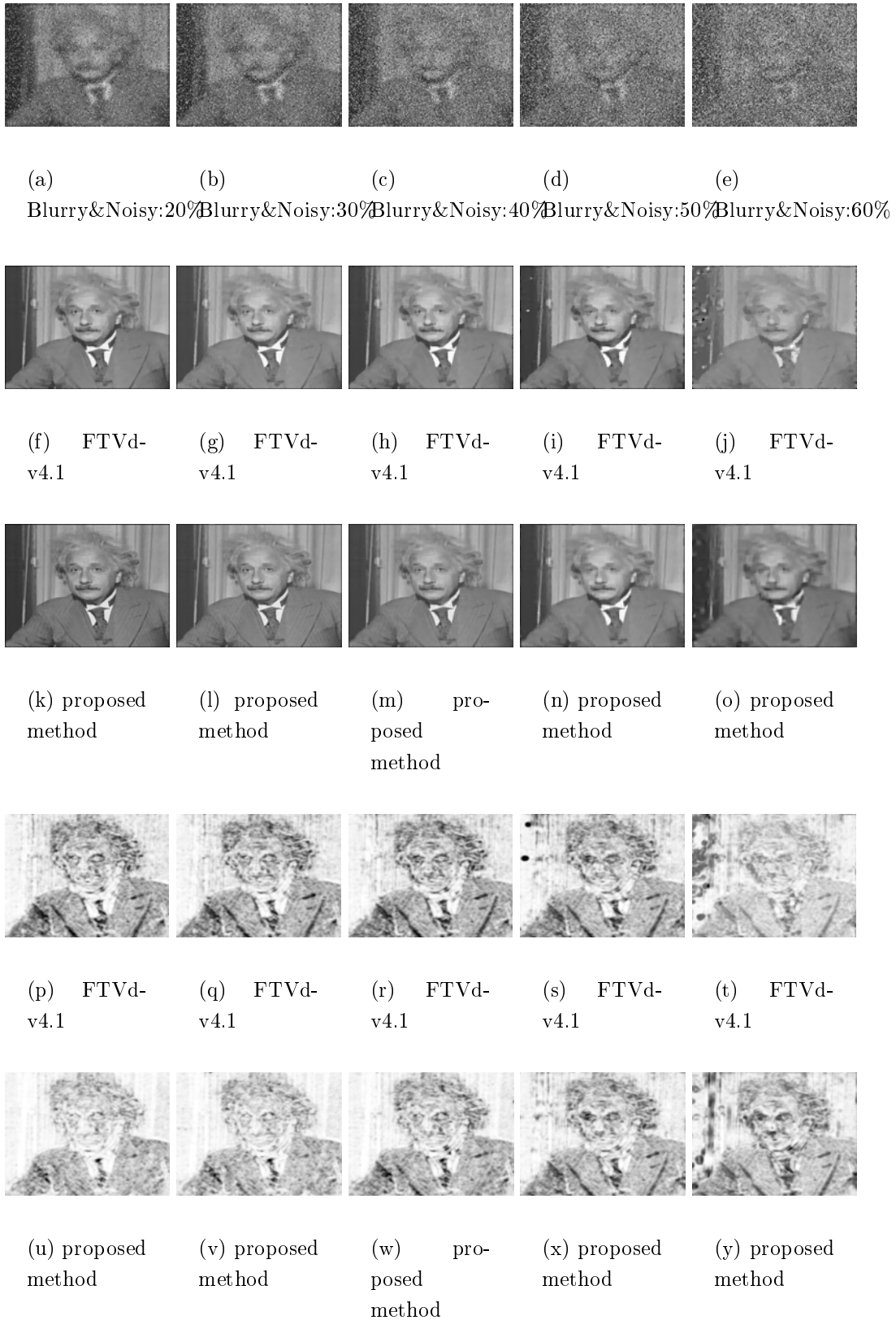
Figure 6: Recovered images of different methods on the Einstein image corrupted by Average(9) and random-valued noise with noise levels from 20% to 60%.
