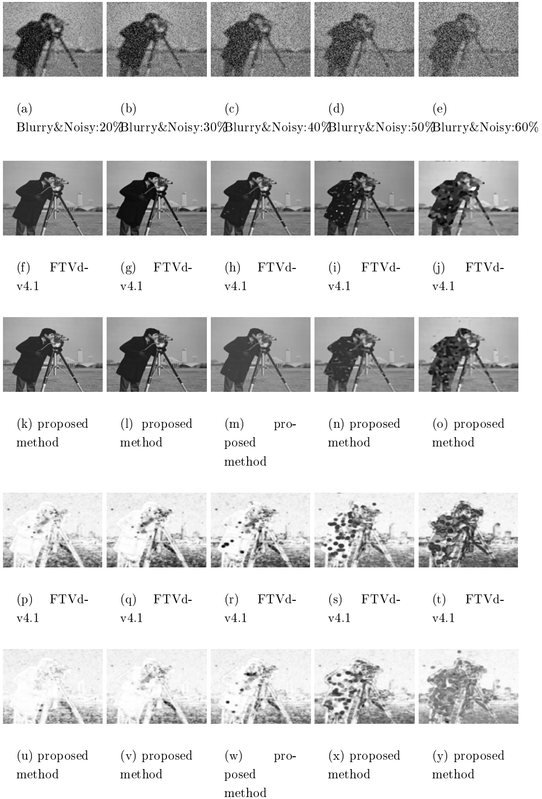
Figure 5: Recovered images of different methods on the Cameraman image corrupted by Gaussian blur G([7, 7], 5) and random-valued noise with noise levels from 20% to 60%.
