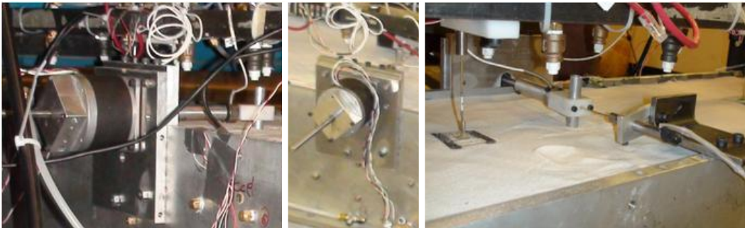
Figure 6: Multiple view of the stepper motor for lateral loading of pile foundation.
