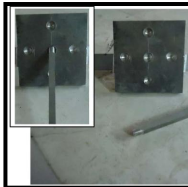
Plate (2): The square aluminum raft model, piles and the screwed opening to fix piles
