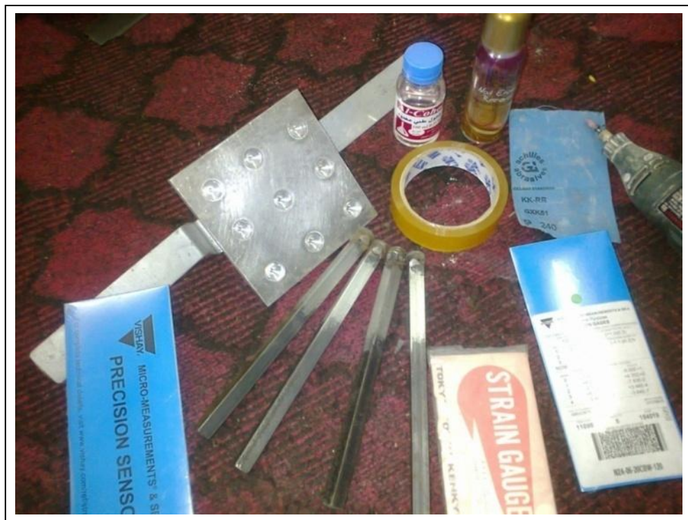
Plate (4): The instrumentation of strain gage
