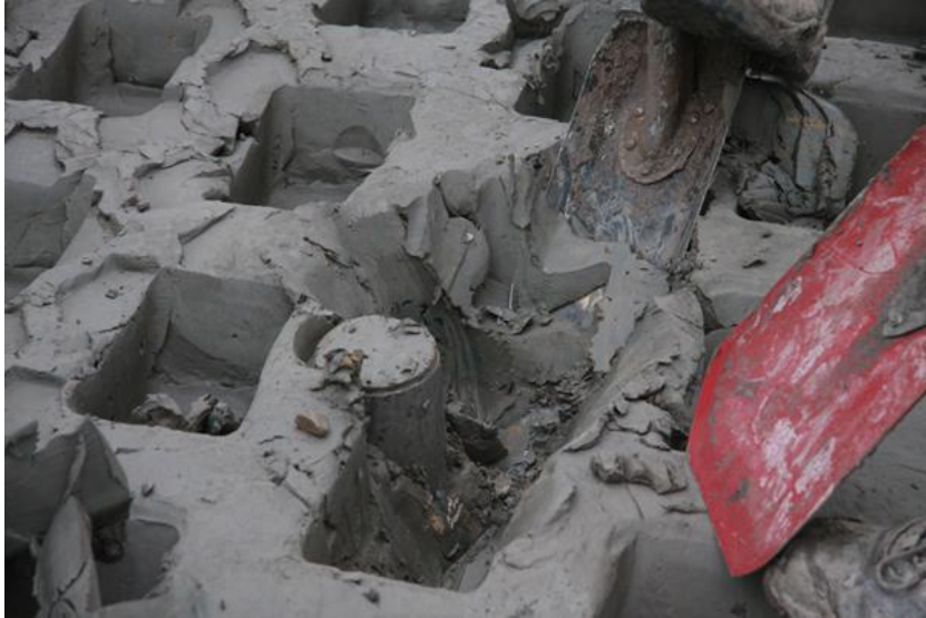
Figure 7: Sampling for determination of water content and density. Notice the homogeneity of the clay.
