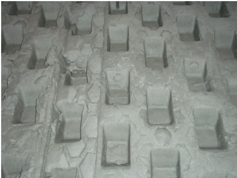
Figure 6: Appearance of padfoot-compacted Friedland clay. The wet surface indicates that the clay was compacted to nearly complete water saturation. It was perfectly homogeneous and no grains or chunks can be seen.
