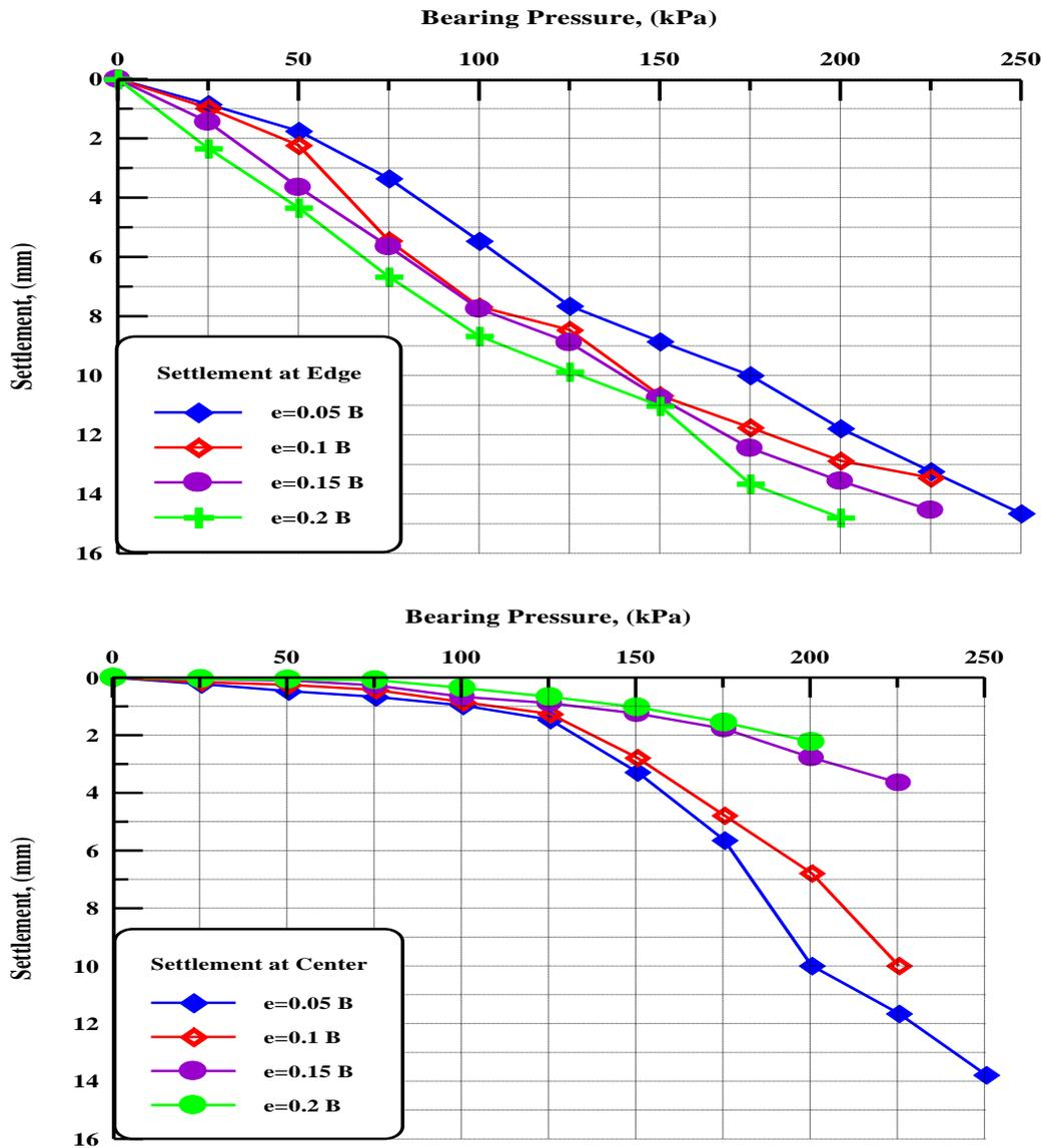
Figure 7: Pressure - Settlement at Edge and Center Curves at Center for Gypseous Soil at Soaked State.
