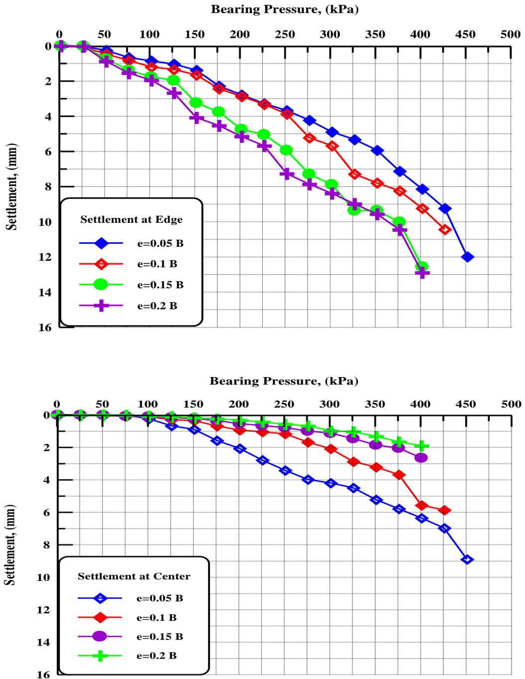
Figure 9: Pressure - Settlement at Edge and Center Curves for Gypseous Soil after Reinforcement on Replaced Soaked Soil.
