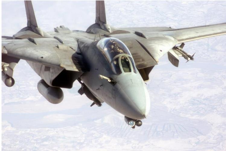
Figure 3: A U.S. Navy F-14D Super Tomcat preparing to connect with a tanker with its refuelling probe out. One can observe under the chin, the AN/AXX-1 Television Camera Set (TCS) and the AN/AAS-42 IRST (with the dark dome). Retired in 2006, this had been until recently the last IRST-equipped U.S. fighter.
