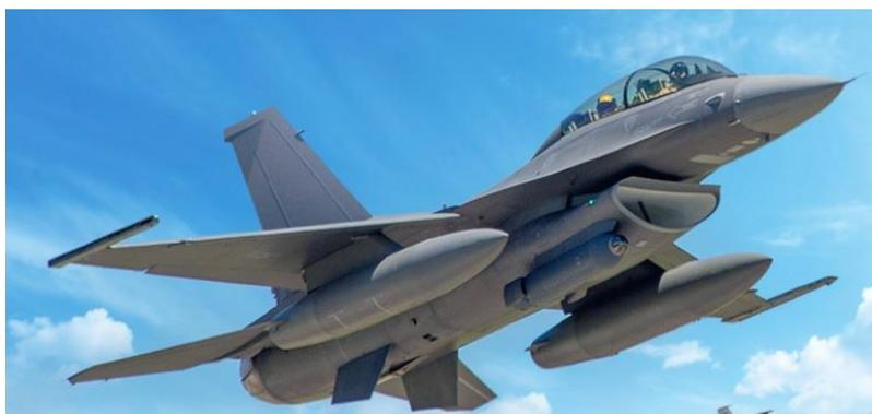
Figure 4: An F-16 equipped with the Legion Pod sensor system. Integration and flight tests have been completed on F-16 (image from the manufacturer's website).
