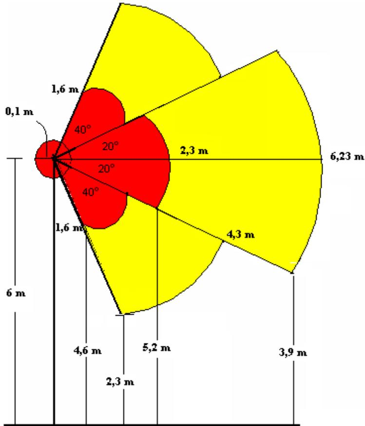
Figure 4: Estimated RF exposure safety zones due to modeling approach
