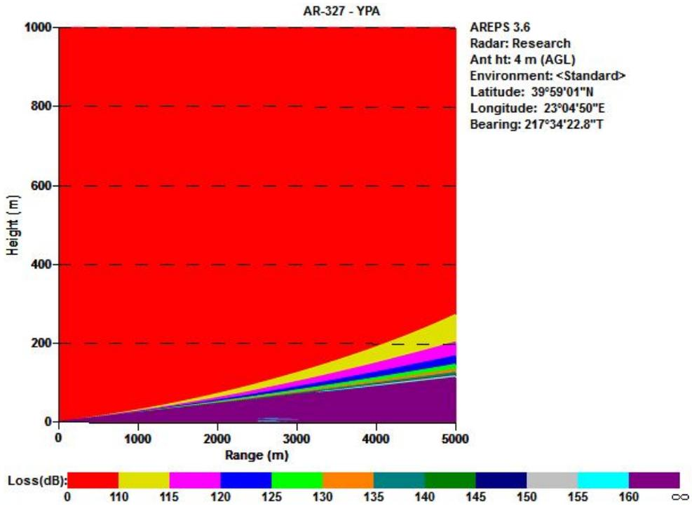
Figure 2: The radio coverage of radar Y before installation of new RADAR
